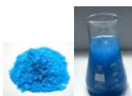
Copper (II) hydroxide Formula: \text{Cu}(\text{OH})_2 Description: Light blue solid, not soluble in water
