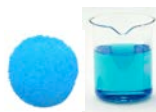
Copper (II) sulfate Formula: \text{CuSO}_4 Description: Light blue solid, soluble in water: aqueous light blue solution
