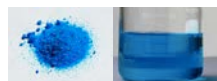
Copper (II) nitrate Formula: \text{Cu}(\text{NO}_3)_2 Description: Light blue solid, soluble in water: aqueous dark blue solution
