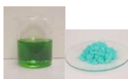
Copper (II) chloride Formula: \text{CuCl}_2 Description: blue-green solid, soluble in water: green to blue aqueous solution
